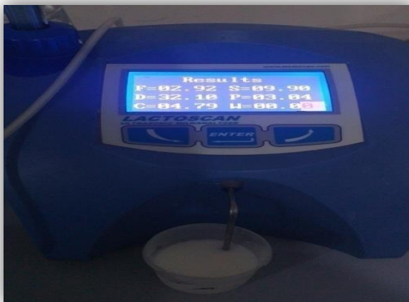
Figure 39. Lactoscan SP Ultra-Sonic milk analyzer.
