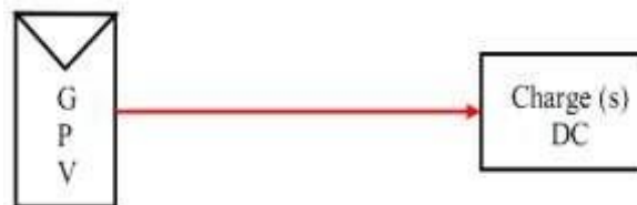
Figure I.17 : Couplage direct GPV-charge.
